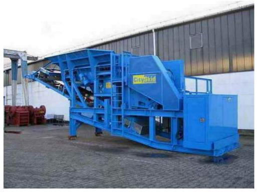
Info: Why always using trackmobile? For user of public power supplier, the CitySkid 960V3/V4 offers some interesting perspectives. On demand, the 24t heavy 900x600 can be loaded via Wolffs Leg on every standard low-loader without using any cranes.
