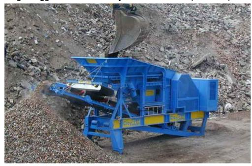
Info: The 700x500mm single toggle jaw crusher can be fed by a wheel loader or an excavator. A smart construated feed opening ensures a failure free processing of oversize and finest grain. Through the 800mm wide discharge conveyor, the grading is getting piled.
