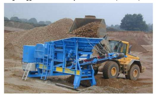
Info: The 920x250 single toggle jaw crusher is able to crush sizes until 250mm to a 0-32mm final product without using a screening plant. This type of CitySkid replaces several of plant combinations as e.g. cone crusher and jaw crusher. The machine is automatically controlled with a filling sensor behind a prescreener or through the feeding of a wheel loader.
